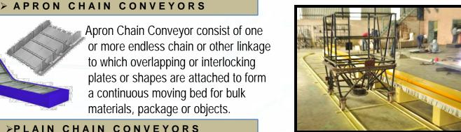
These have chains with attachments or lugs fastened to the chain at intervals so they may push various objects which slide or roll on their own surfaces. This type is used to handle buggies, tote bins, billets plates,
