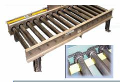
Chain Driven Powered Roller Conveyors (commonly referred to as pallet conveyors) are the more heavy duty and robust of the roller conveyor range, and are used in such instances as pallet handling, adapted for loads of (usually) 1,500kgs, but can easily be adapted to handle loads of up to 7,000kgs.
