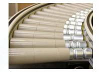
Line shaft roller conveyor is a powered conveyor system. It has the capability of accumulating products with minimum back pressure. Typical characteristics include quiet operation and easy maintenance. Suited for many applications, including: side loading conveying, smooth merges and low pressure accumulation application conveying
